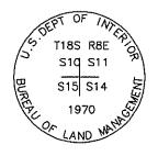
0818300500 NW COR S 14 T18S R8E SLM STD. BLM CAP
