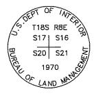
0818500400 NW COR S 21 T18S R8E SLM STD. BLM CAP
