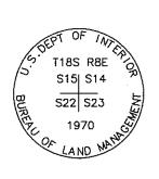
0818300400 NW COR S 23 T18S R8E SLM STD. BLM CAP
