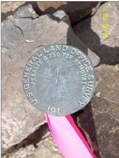
Corner Monument Markings - Photo View or Stamping on Cap
