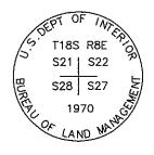
0818400300 NW COR S 27 T18S R8E SLM STD. BLM CAP
