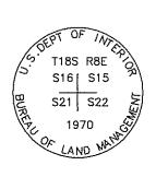
0818400400 NW COR S 22 T18S R8E SLM STD. BLM CAP
