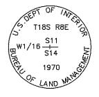
0818260500 WEST 1/16 S14 T18S R8E SLM STD. BLM CAP SET #5 REBAR N 14'30'0'
