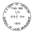
0818300440 WEST QTR S 14 T18S R8E SLM STD. BLM CAP SET #5 REBAR S 84\*47'36" W , 9.80
