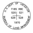
0818500300 NW COR S 28 T18S R8E SLM STD. BLM CAP
