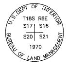
0818500400 NW COR S 21 T18S R8E SLM STD. BLM CAP
